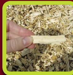
To ensure that the chips comply with the specifications, Clare Wood Chip Ltd takes a sample of approximately 2.5kg from each load, which is sent for independent testing. The moisture content of the sample is determined using the oven dried method. The sample is then sieved using a grader. The proportion of over sized pieces and dust is determined as a percentage of the total weight of the sample. A hard copy of the results is provided to both the supplier and end user.
